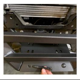
Attach the Winch Plate to the bumper using the included 3/8" carriage bolts and nuts.
