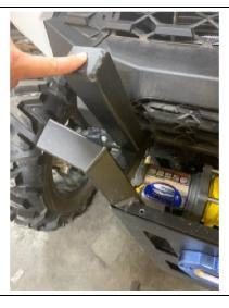
11. Attached with provided bolt and nut to the tube bumper.
