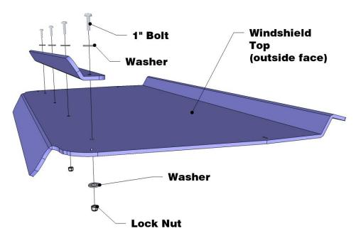
5. Now you are ready to place the windshield on the Ranger and attach to the roll cage. **NOTE: THE BEND AT THE TOP OF THE WINDSHIELD SHOULD GO BELOW THE TOP TUBE**. The diagram on the next page shows the proper placement for the hardware. Install the clamps as shown for the top two slots in the windshield only. Use the 1" bolts for this application.
