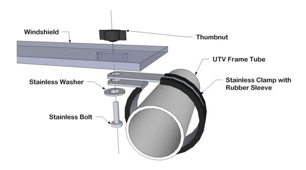
6. Now Place the two halves onto the frame as shown below.
