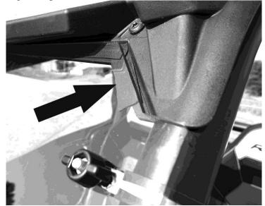
7. You are now ready to install the windshield on your roll cage. Place the windshield on the vehicle first. Then take the four Velcro clamps and place them through the square holes then wrap the strap around the roll cage and under the wire as shown in the photo below.
