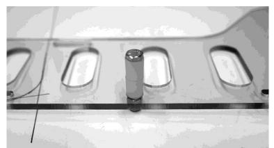
Now insert the bolt in the small holes and screw on the lock nuts so the end of the bolt is flush with the outside edge of the lock nut. No need to worry about which side to install the handles on, it works both ways.
