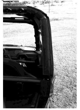
5. Lastly snap the bottom of the door to the plastic doors on the RZR. NOTE: it helps to place the screw snaps into the sockets on the cabs first, then starting at the top one, push them into the plastic so a small dimple is left behind. Then pull the screw snap back out and screw it into the plastic where the mark was made. See photo below
