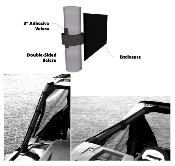
4. After installing the double-sided strips move to the rear of the door and attach the two Velcro tabs to the rear bar using the corresponding adhesive Velcro strip. See Photo Below:
