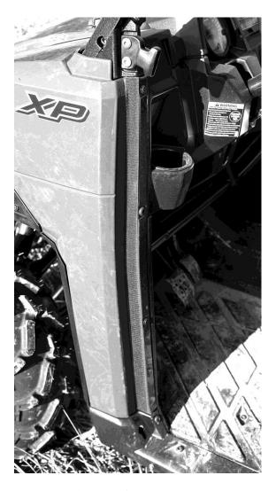
10. Last step is to install all of the snaps along the bottom of the doors. It works best to put the screw studs into the snap sockets on the door first. Then one by one pull the door in place and push the screw into the plastic making sure to put enough pressure to leave a mark. Then remove the screw stud from the door and install it where the mark was left behind at. The following pictures show where all the snaps should be placed.
