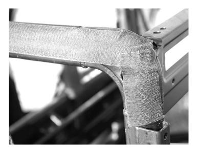
8. Next place the 20" strip down the back of the cage as shown in the photo below.
