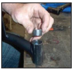
Reinstall the bushings, sleeves, and pivot caps into the new arm.
