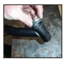
NOTE: APPLYING GREASE TO THE BUSHINGS AND SLEEVES WILL MAKE THE INSTALLATION EASIER.
