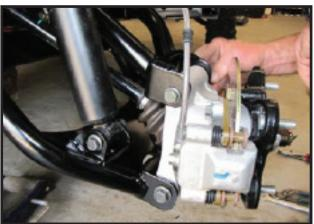
Attach the lower arm to the hub assembly using factory hardware. DO NOT FORGET WASHERS.
