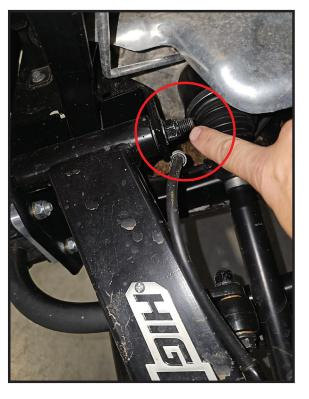
Once bushings are installed, connect the new upper arm to the frame using the factory hardware. DO NOT FORGET WASHERS.
