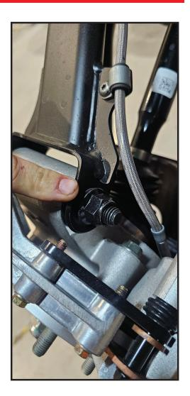
When all arms are removed, install the Sway Bar spacers. (before installing new arms) Remove the 4 bolts holding on the sway bar support, 2 bolts on either side. Slide new spacers against the bar. Install new bolts, washers and locknuts included with your kit.
