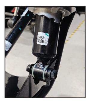
Connect the new lower arm to the frame and the lower portion of the shock using the factory hardware.
