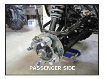
Place jack under the rear center of the UTV and lift until the weight is off the suspension.
