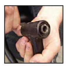
Use caution when removing the bushing from the collar, there is a stop built into the factory arm that prevents the bushing from pushing out when installed. Because of this, the bushing must be pushed out from the opposite side! A flat punch is recommended to remove the bushings.
