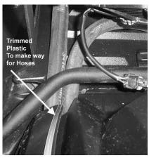
11. Mark the areas that need to be cut. Start with a small area and expand if needed. The Dash Board and the Central Panel are easy to take on and off, so if you need to cut more it is easy to do.
