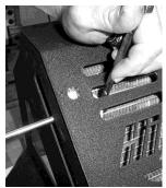
10. Once the kit is assembled, place the kit on the front rack and mark the holes for the water lines that need to be cut. We chose one location to route our lines. There are many different ways to run the lines, we chose what we thought was the easiest way. See finished illustration.
