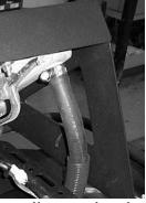
15. Connect the ¼" black overflow hose to the radiator and to the overflow bottle line. Use the ¼" hose barb and ¼" black hose to extend the overflow bottle hose to the radiator neck. Use zip ties to secure the hoses. **NOTE: In our photos we used clear hose, for production we used black hose.**
