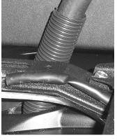
14. Connect the hoses to the radiator using the clamps provided in the kit.
