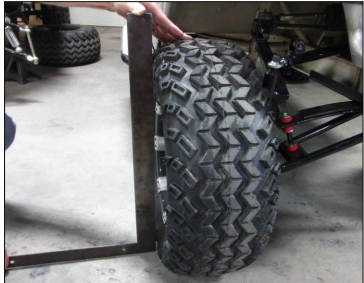
Front camber setting should be set using a square as shown
