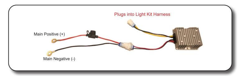
The voltage converter included must be used on all carts electric and gas. Connect the red wire with the fuse to the Main Positive terminal of the battery pack. Connect the black wire to the Main Negative terminal of the battery pack and tighten hardware.
