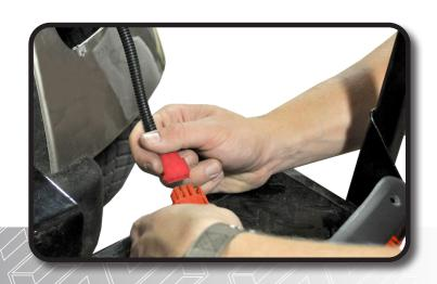
Install new tail lights using retained hardware.
