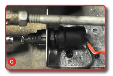
Mount Turn Signal Indicator assembly using clamps provided and tighten. Run Turn Signal Indicator harness along steering column and insert harness through dash.
