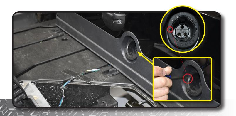
Remove the screws securing the lower body trim to the body. Retain hardware. Remove the lower body trim.
