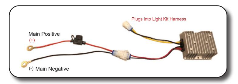
The voltage converter included must be used on all carts electric and gas. Connect the red wire with the fuse to the main positive terminal of the battery pack. Connect the black wire to the main negative terminal of the battery pack and tighten hardware.
