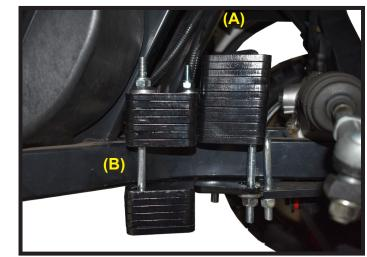
**NOTE:** If you intend to use two 16-058 kits (60 total lbs) on a Yamaha G29/Drive2 you will use the setup shown below on each side of the front frame. For E-Z-GO RXV, you can use either option listed above due to the extra mounting space available vs the Yamaha models.
