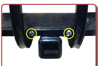
Attach receiver with supplied pin clip to complete installation.
