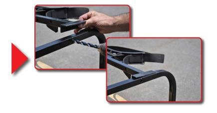
Line up Golf Bag Attachment Bar assembly with hole and fasten to armrest with threaded knobs.
