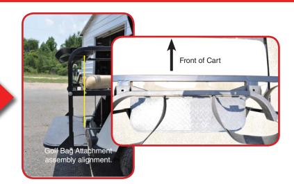
Align a straight edge with the center of the welded in nut on the Golf Bag Attachment Bar and mark the outside of the armrest. This will be the center of where you drill.
