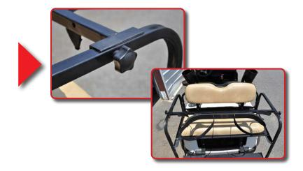
Route Lower Securing Strap around bag well brackets and fasten
