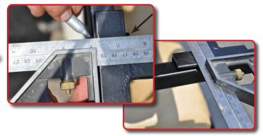
Strike a vertical line on the armrest to mark drill location. Using a 11/32 Drill bit, drill through armrest.
