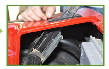
Insert Main Brackets into holes where OEM front seat supports were removed. Be sure the tabs are pointed to the cart's CENTER, as shown. Secure the Main Brackets with hardware retained in step 6.
