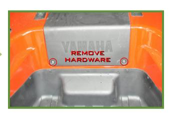
Remove OEM front seat supports. Retain hardware.
