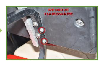
Remove OEM front seat backs. Retain hardware. STEP 3
