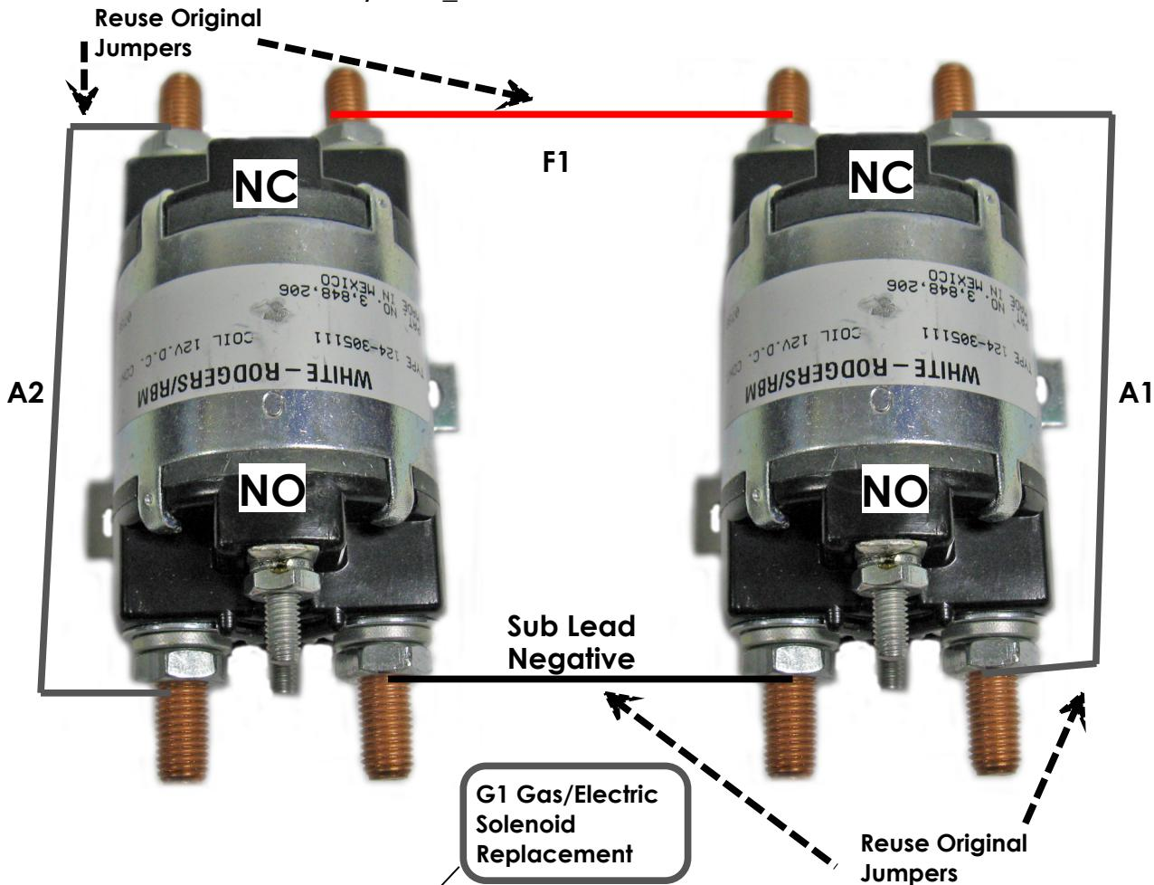
The O.E.M. solenoid contacts are opposite to the new replacement. The old style has normally open (NO) contacts on the two pole end. The four pole end is normally closed (NC).
