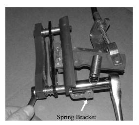
Fig R7 – Caliper re-assembly
