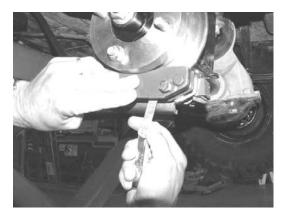
Fig. R8 - Check pad clearance
