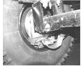
Fig 15 – Brake inside wheel
