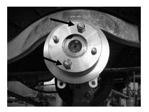
Fig R3 – Install 2 lug nuts.
