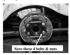
Fig 2 Original drum brake assembly
