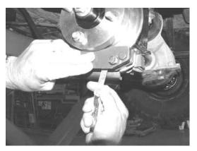
Fig. M4 Check pad clearance of both wheels at the same time.
