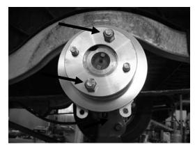
Fig. 6 - (2) lug nuts to temporarily hold rotor in place.
