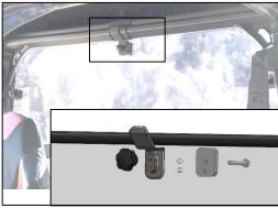
8. Attach the half clamp with bolt and knob as shown above. Tighten knob to secure panel.
