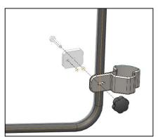
6. Line up holes in the backing plate with holes in the panel and insert. The peg on the backing plate should go in the inside holes (not the holes near the edge of the panel).
