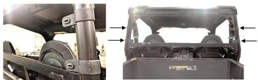
4. Open the clamp and place around roll cage with the SZ logo facing backwards as shown.
