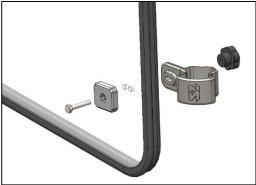
**7.** Attach the rear panel to clamp with bolt and knob as shown above. Tighten knob to secure panel.
