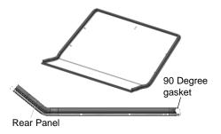
3. Push the 90 Degree gasket on the three other sides of the panel. Make sure the bulb edge is on the **inside** of the bend.
