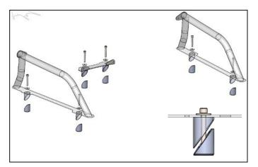
**3.** Attach the wedge nuts to the two basket side supports and center basket support using (6) M8x60mm bolts. Tighten just enough to hold the wedge nuts on.
