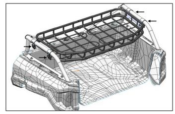
**8.** Secure the basket with (4) star bolts. Make sure to tighten all bolts before use. There are 6 securing the basket supports to the bed, and 4 securing the two support rods to the basket assembly.
