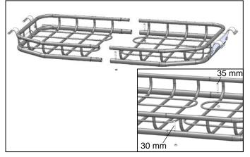
1. Assemble the two sides of the basket by first pushing the left side of the basket into the right side of the basket. Secure with a M6 x 30mm and M6 x 35mm button head bolts and M6 locknuts. The longer bolt goes in the back of the basket.
