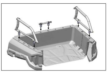
**4.** Place the three pieces from step 3 into the holes on the top edge of the bed rack.
