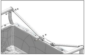
**5.** Attach the support rods with (4) M8 x 35mm Hex bolts (8) M8 washers, and (4) M8 Locknuts. Hand tighten bolts, but do not snug yet.
