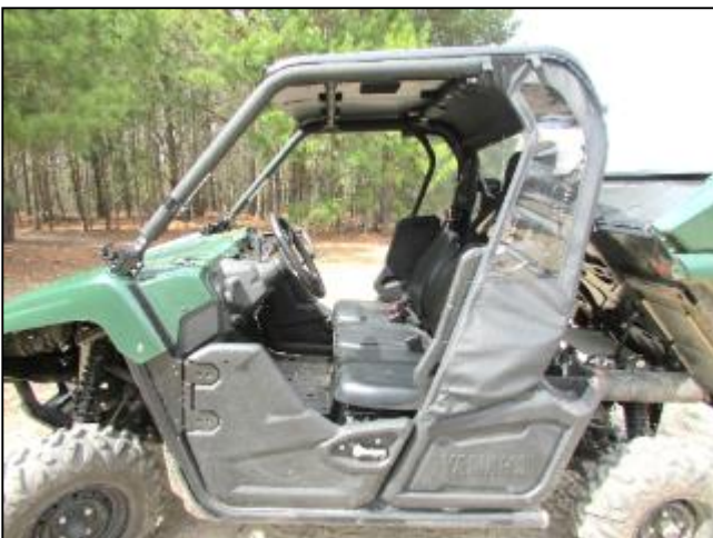
13. Secure the back panel around the Z tube. If needed, refasten the Velcro straps to adjust the fitment of the textiles.
