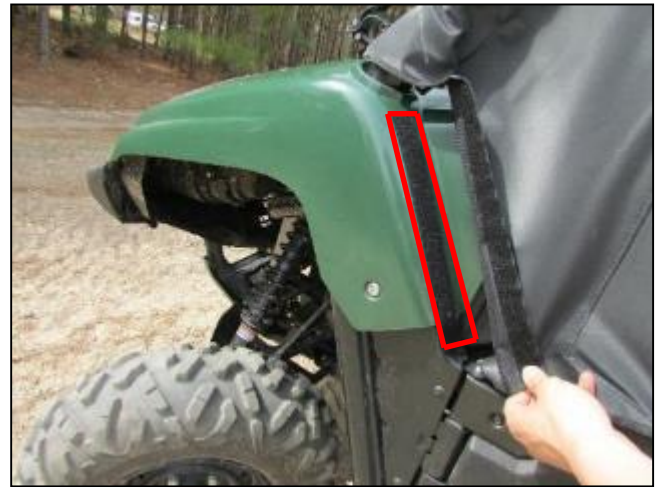
22. Attach a strip of Velcro on the back side of the cab on the lower crossbar. Attach back panel lower flaps.
