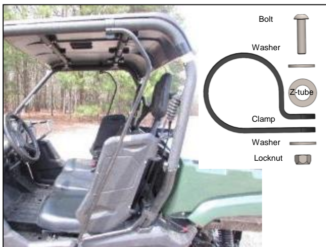
7. Attach the Z tube to the side of the vehicle with a M6 x 35mm button head bolt on the top clamp and a M6 x 25mm button head bolt on the bottom clamp. Use 2 washers between the plastic clamps and nuts.
