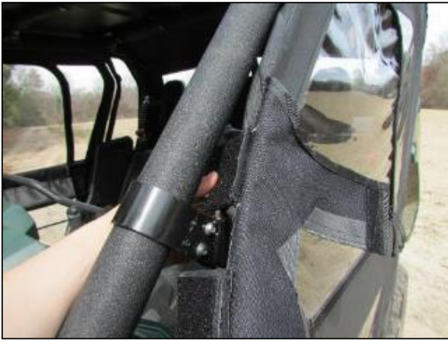
21. Secure the remaining flaps on the front roll cage bar of the vehicle. If needed, refasten the velcro straps to adjust the fitment of the textiles.
