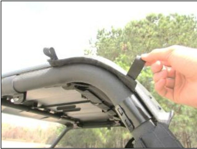
15. Pull the loop through the side of the vehicle between the roll cage and roof.
