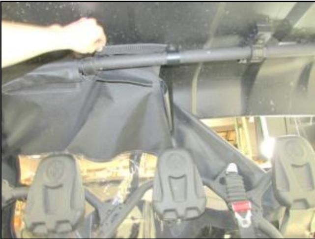
11. Slip the top four flaps of the back panel between the rear upper crossbar and the roof and attach.
