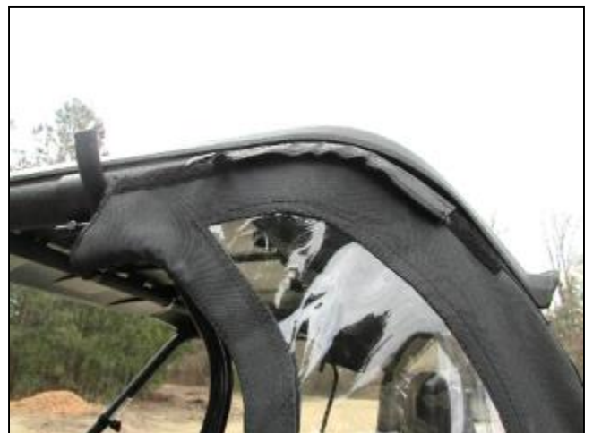
14. Match the velcro strip near the loop and velcro on the flap and attach.
