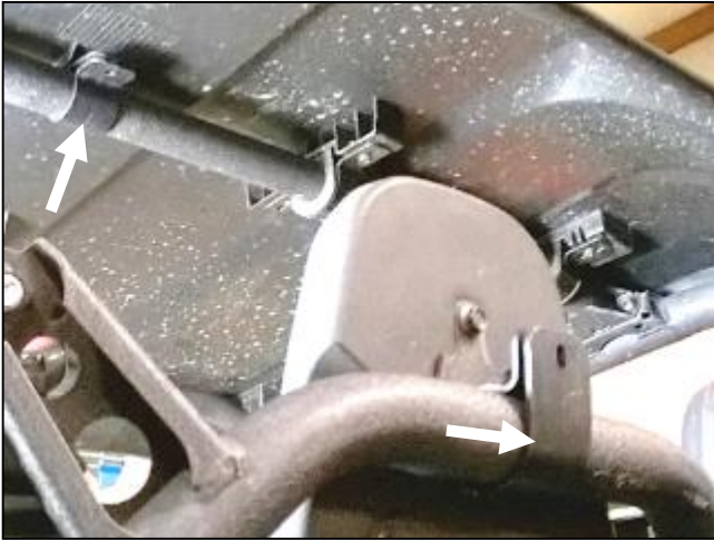
9. Attach a plastic clamp on the rear bar behind the center headrest. Attach a clamp on the rear upper crossbar as shown above.
