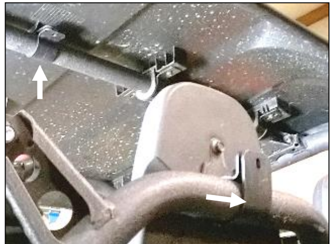
6. Attach a plastic clamp on the rear bar behind the center headrest. Attach a clamp on the rear upper crossbar as shown above.
