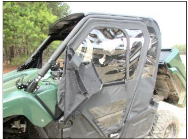
18. Place Seizmik door on OEM Viking door and roll cage barrel clamp. Adjust position of the door and tighten the roll cage barrel clamp bolts.
