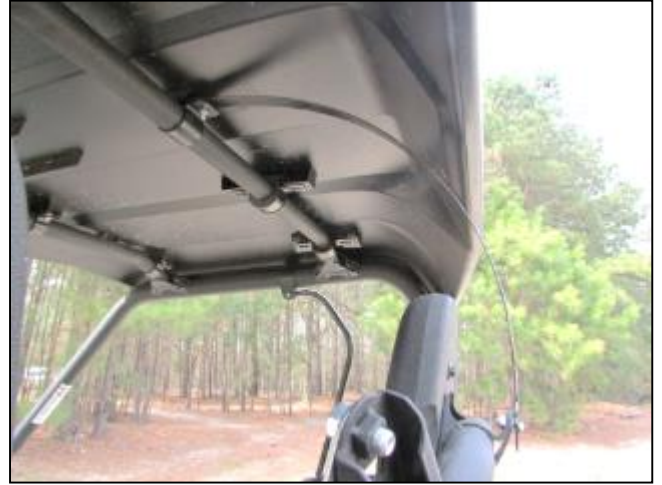
10. Attach the aluminum rod onto the top clamp with a M6 x 25mm bolt, nut and washer. Bend the rod down and attach to the other plastic clamp with a bolt, nut and washer. Make sure the bolts face inward to avoid puncturing the textiles.
