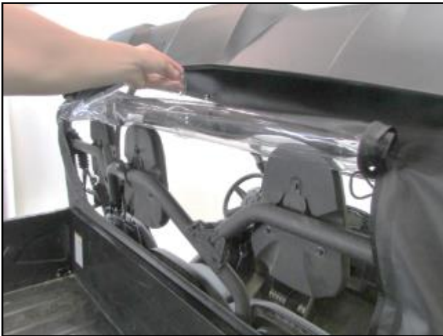
23. To roll up the back window, unzip the vinyl section and roll up. Use the vinyl straps to secure the rolled section.
