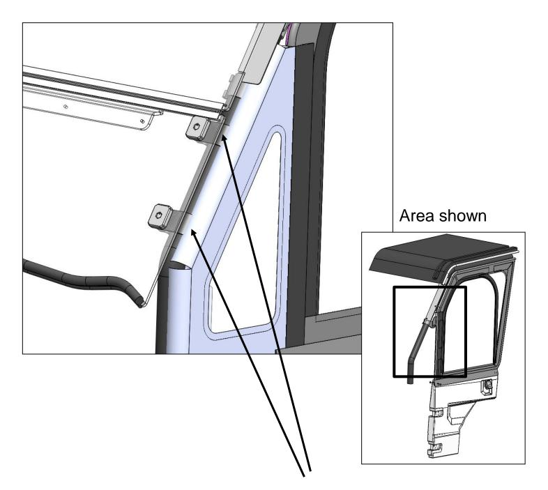
Because there are so many different windshields, you will have to cut the front textile for whatever clamps your windshield uses. Set the windshield in place over the installed textiles, and using the mounting holes in the windshield as a guide, mark the clamp locations on the textile. Using a sharp knife, cut slits in the textile for the clamps and install the windshield.
