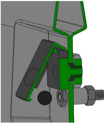
4. Insert the pushrod and knob back into the threaded tube from the inside and screw the knob onto the other end. The thin nut should still be flush against the threaded tube to leave as much room as possible for the knob under the paddle. Tighten both knobs.
