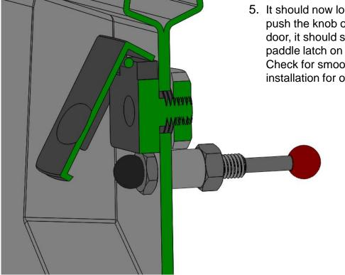
It should now look like this. When you push the knob on the inside of the door, it should smoothly operate the paddle latch on the outside of the door. Check for smooth operation and repeat installation for other door.
