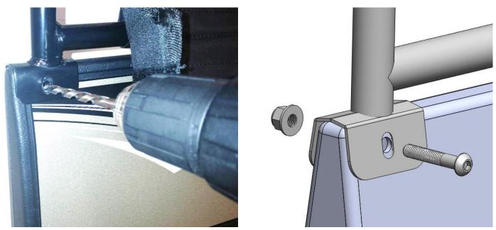
2. When you are satisfied with the fit, Use the brackets as a guide, carefully drill a 1/4 hole through the door in the front and rear locations. Bolt door in place using the M6x35 bolt in the front, and the M6x40 bolt in the rear. The nuts should be on the inside of the door. Repeat for other side.
