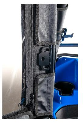
**13.** Locate the mirror mounting bracket on the inside of the door frame. Mark the location of the hole with a punch so that it can be seen on the outside of the door textile.
