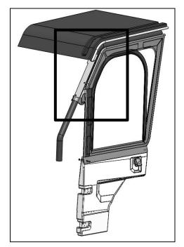
Begin by snapping 2 plastic P clamps onto the roll cage in the locations shown. The flanges should face the front and towards the outside of the vehicle. Bolt the plastic gutter in place as shown using M6x20 bolts and nuts. The upper part of the gutter should go under the front edge of the roof. Angle the gutter down slightly so the water will run away from the vehicle instead of onto the windshield.
