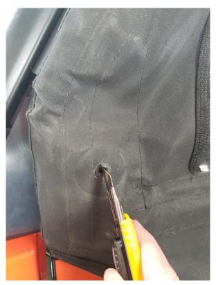
**14.** Using a sharp razor or utility knife, cut the textile so the mirror mounting bolt can pass through.
