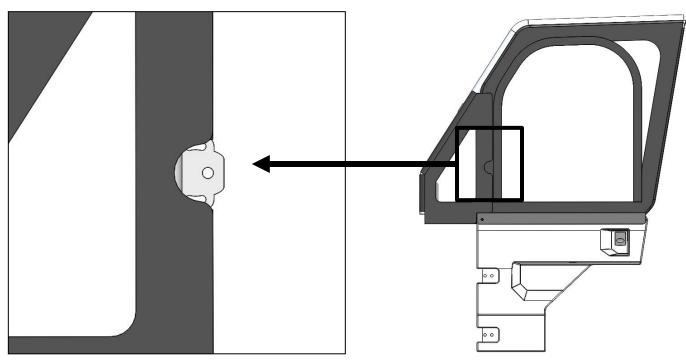
2. The half round cut out in the filler panel should also be centered over the mirror bracket welded to the front tube of the door frame. When everything is lined up, fold the front filler panel flaps around the roll cage tube and fasten to the Velcro on the opposite side. Re-adjust as necessary for best fit. Repeat for the other side.
