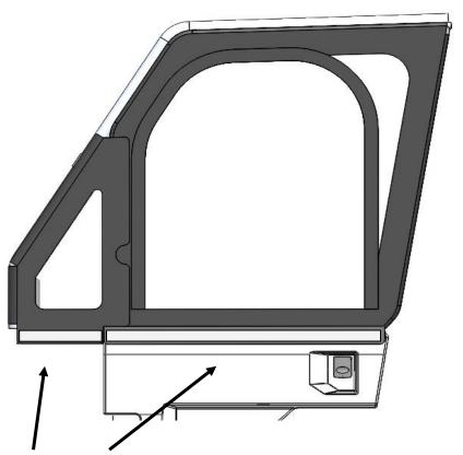
When you are satisfied with the fit of the door and filler panel, locate the strips of self adhesive Velcro on the back side of the textiles in the locations shown. Clean the areas of bodywork underneath them thoroughly using rubbing alcohol. Peel off the protective backing and press them down firmly on the bodywork.
