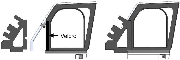
1. The door should be shut and latched for this next step. Install the filler panel textile by first attaching it to the 2" Velcro on the front edge of the door. The bottom should line up with the bottom of the flap on the door.
