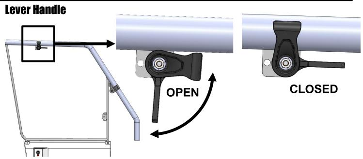
Because the factory door is so short and requires such a tall upper door to close the cab, it requires a little extra to hold it closed tightly. You may choose not to use this while riding but it is recommended for trailering the vehicle. When inside just rotate the handle forward to close the door tightly. If trailering, unzip the window from the outside, turn the handle, then re-zipper the window.
