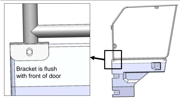
1. Place metal door frame on the plastic factory lower door. Position frame making sure the bracket on the lower front is flush with the front of the lower door as shown
