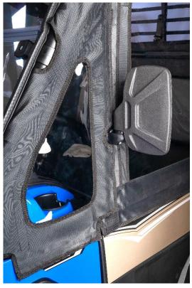
**15.** Pass the bolt through the mounting bracket and thread into the mirror and tighten (DO NOT OVER TIGHTEN).
