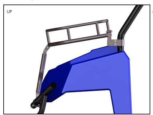
**8**. To fold down the hood rack, simply remove the rear U-clamps and stargrip bolts, and pivot the assembly forward and down.
