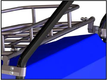
**6.** Have an assistant hold the front of the assembly while you set the basket arms down onto the rear clamps, as shown.
