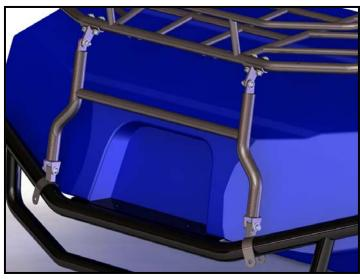
8. Set the bumper clamps down onto the bumper.
