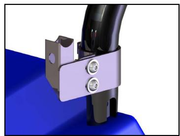
5. Install the driver-side roll cage clamp, setting the bottom of the clamp immediately above the weld bead on the cage tube. Orient the assembly so the tube portion is pointing forward. Bolt through the clamp arms as shown, using the M8 x 30 bolts, washers and nuts.
