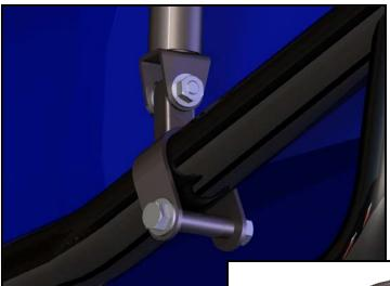
**9.** Secure the bumper clamps with the 3/8" bolts, washers and nuts, sliding a crush sleeve between the two clamp halves as shown.
