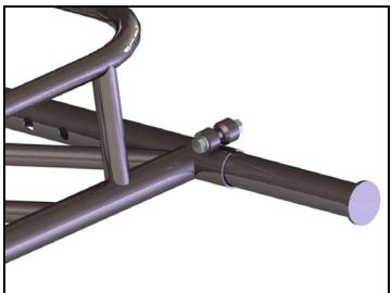
1. Slide the basket extension arms into the long receiver tube at the rear of the hood rack basket. Insert the M6 hardware through the two welded bosses as shown, and leave slightly loose for now. Repeat for the other side.
