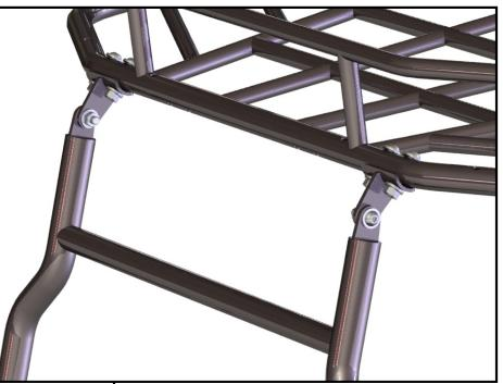
4. Attach the bumper clamps to the bottom of the front riser, as shown. Bolt through using M8 x 45 bolts, washers and nuts.
