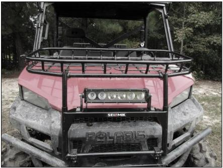
Lights or a light bar can be attached to the hood rack by drilling holes in the light mounting plate. We recommend our 13" 60 Watt Siezmik Light Bar with 5,400 Lumen output. Part Number #12037
