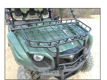
**3.** Open the four clamps on the vehicle. Lift the entire hood rack assembly onto the four clamps.
