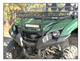
Lights or a light bar can be attached to the hood rack by drilling holes in the light mounting plate. We recommend our 13" 60 Watt Siezmik Light Bar with 5,400 Lumen output. Part Number #12037
