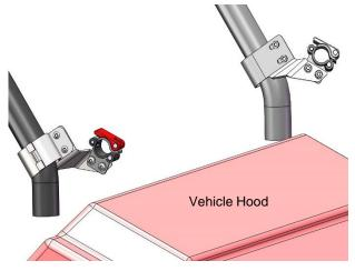
1. Attach the roll cage clamps with two M6 x 16mm bolts, nuts and washers. Attach two clamps with two M6 x 16mm bolts, nuts and washers. Make sure the top clamp lever opens towards the front of the vehicle.
