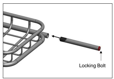
2. Insert an Extendable Tube (B) in each end of the hood rack. Push in just a few inches and tighten the locking bolt in the end of the tube just enough to hold the extending tube in place. You will make a final adjustment and tighten later.
