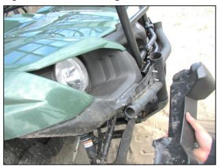
1. Remove plastic bumpers. There are two selftapping screws and one machine screw on each side. Look for the machine screw under the fender.
