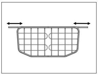
**2**. Adjust the position of the extendable tubes so they stick out just past the clamps.
