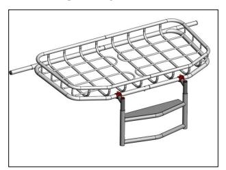
1. Attach the front assembly to the hood rack.
