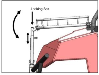
**5**. The hood rack angle can be adjusted by loosening the bolt on the front riser stems and lifting up or pushing down on the front of the rack. Adjust clamps and brackets as necessary, then tighten all bolts.
