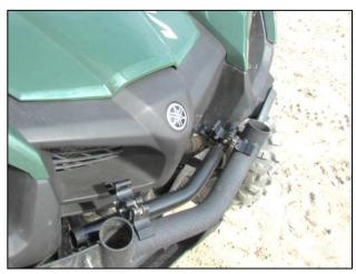
**3.** Install two clamps on the bumper mount using the M6 x 16mm bolts and nuts.
