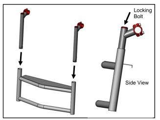
2. Insert the riser tubes into the Front riser/Light Mounting Plate. The flanges on the tubes should face toward the light mounting plate. Tighten the locking bolt at the top of the tube just enough to hold the riser stems in place. You will tighten after final assembly.
