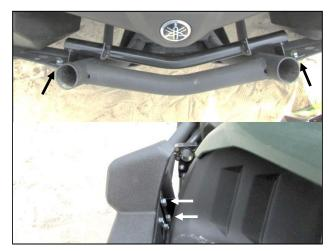
2. Install the bumper mount using four M8 Hex head bolts and nuts.
