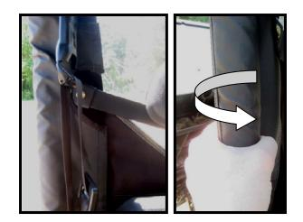
2. Locate the straps running down the length of the rear vertical ROPS bar. Fasten around the bar. Repeat this step for the opposite side. A good way to get the straps tight is to rotate the top around the bar like in the picture on the right.
