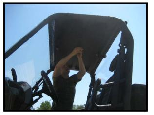
3. The last step is to fasten and pull tight the (3) roof straps. Some adjustment may be necessary to ensure a proper fit.
