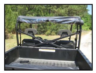
A - The rear window can be rolled up by undoing step 3, rolling the window up from the bottom, and securing with the three straps at the top of the window as shown.
