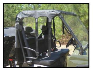
1. Lay the soft top over the roll cage of the vehicle making sure the straps are on the outside of the roll cage. Lift the dump bed to make installation easier.
