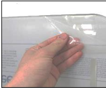
1. Peel plastic 4" back on bottom of windshield. Remove completely after windshield is fully installed.
