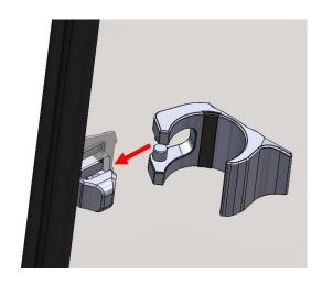
The Seizmik Toolless Clamps should come fully assembled on your windshield. It is possible that one or more of the clamps could come apart during shipping. If this happens simply put the base back through the hole in the windshield, then snap the clamp back into the slots in the base
