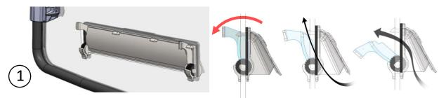
This vent has multiple detents to hold the position of the flap. Open ONE click for Defog, after that, adjust to suit.
