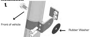
Disassemble clamp by removing the two 8mm socket head bolts. Place curved half of clamp against roll cage in desired mirror location. Insert bolts and thread into clamp plate with the welded nuts facing the bolt heads. Assemble loosely.
