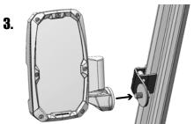
Bolt the mirror to the clamp but do not fully tighten yet.
