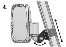
Slide mirror up or down Roll Cage tube to desired location. Rotate mirror on clamp to desired angle. When you are satisfied with the location and angle, tighten bolt.
