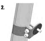
Put mirror mounting bolt through hole and place large rubber washer on the end of the bolt.
