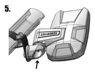
To tighten the folding feature of the mirror, tighten tension adjustment nut on the bottom of the mirror arm.
