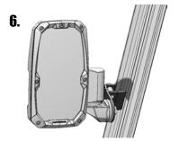
Make the final adjustments and fully tighten mirror mounting bolt.
