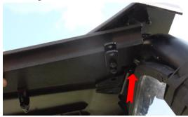
5) Remove outer plastic panel from the inside of the door by removing 6 screws (see photo next column)
