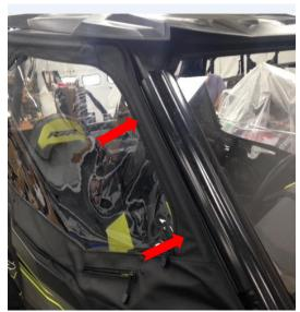
TIP: The OEM door may need to be adjusted forward and backward to create a seal on the ROPS, ensure the front triangle creates a good seal.
