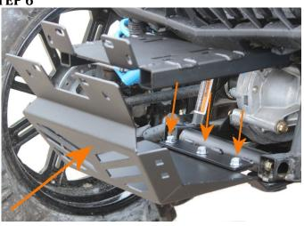
• Install the Bumper Skid Plate using the 3/8 x 1" Hex head bolts and Nylock nuts.
