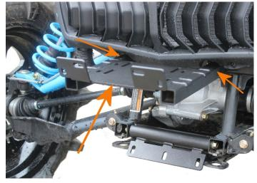
• Using the two upper factory bolts, install the Winch Plate.
