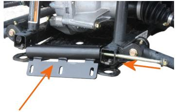
• Install the Bottom Bracket using the longer factory bolt as shown here.
