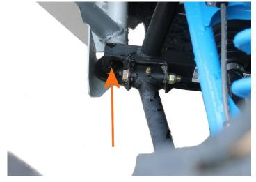
• Remove and retain the longer bolt from the bottom of the bumper.
