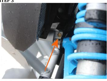
• Remove and retain the remaining upper bolts, from both sides of the bumper.
