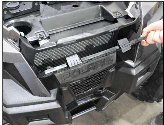
Figure 3: Top Grille Removal
