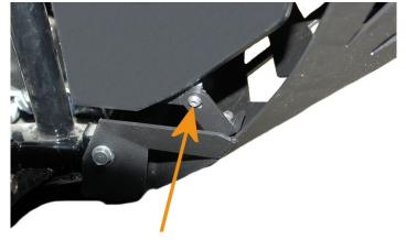
• Use the Factory Bolt removed from this spot to secure the plastic to the bracket.
