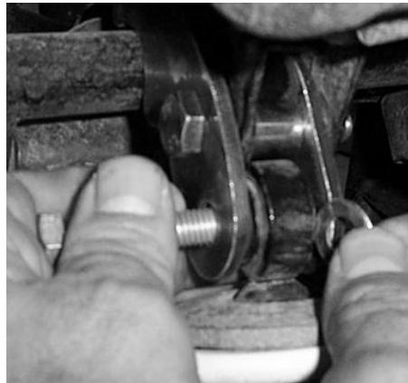
7. Secure brackets using at 10mm lock nut provided in the kit.
