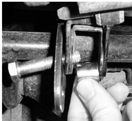
5. Next insert the smaller rear bracket between the spacer and the inside of the shock mount tab.
