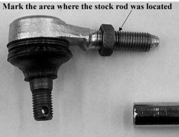
3. Once you have marked both tie rod ends remove the stock tie rod and ends from the ATV.
