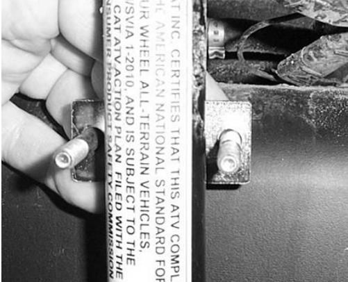
4. Connect the name plate to the backing plates using  $\frac{1}{4}$ " washers and  $\frac{1}{4}$ " lock nuts.
