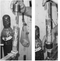
5. Place the stock spring(s) back onto the shock.
