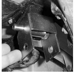
5. Insert the small spacer and top of the shock in the bottom of the lift racket.
