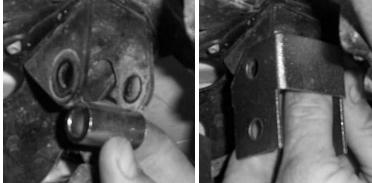
4. Secure the bracket and spacer using a 10x60 hex bolt and 10mm lock nut.
