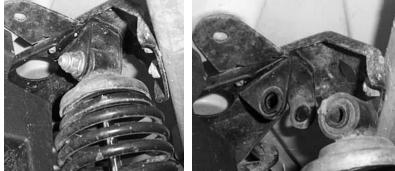
3. Install large spacer and front lift bracket into the upper stock shock mount location.
