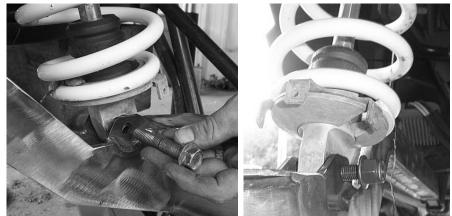
11. Connect the rear knuckle assembly and rear radius bars to the new trailing arm using the factory hardware.
