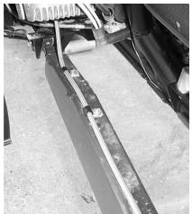
5. Disconnect the caliper/knuckle/hub assembly and radius bars from the factory trailing arms.
