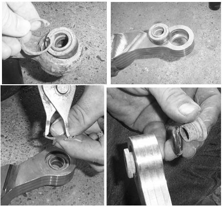
9. Once you have installed the factory bearing, bushings, seal and retaining clip, connect the new trailing arm to the frame using the stock nut and bolt that held the factory trailing arm in place.
