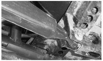
8. Once you have removed the arm, you will need to reuse your factory spherical bearing, bushings, seal, and retaining clip located in the factory arm. We recommend that you check it for wear. Now insert all into the new High Lifter Trialing Arm.
