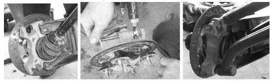
12. Next attached the factory sway bar link to the new trailing arm using the 10x55mm bolt and 10mm lock nut provided. Make sure it attaches to the inside of the trailing arm.
