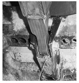
10. Connect the shock to the new trailing arm using the factory bolt and lock nut.
