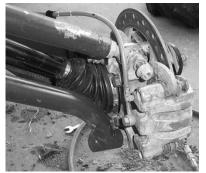
14. Attach the P-clamp to the trailing arm, making sure the brake line does not get pinched or cut during operation. There are predrilled holes in the arms to attach the P-clamps and you attach them using the #10-3/4" Tek self-tapping screws.
