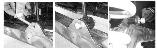
13. If you have done so already, attach the brake caliper and brake lines to the new trailing arm by using the factory P-clamp, additional P-clamps in the kit and Self-tapping screws provided into the holes already predrilled in the arms.
