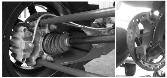
6. Next, disconnect the arm from the shock at the shock mount point. You will need to remove the shock dust shield from the shock. It will not work in conjunction with the new arm.
