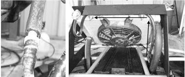
24. Connect the overflow vent line to a location that will not allow the overflow to spray on the rider. We connected ours to the front of the rack. Use a zip tie to secure the hose.
