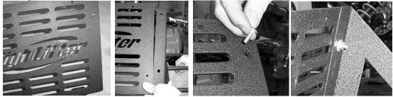
7. The bottom of the stock radiator has two rubber grommets that you will need to place in the holes at the base of the new face plate. They may still be attached to the frame and did not come out when you removed the radiator.
