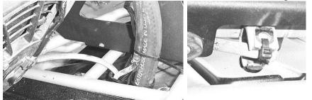
25. Using the blue butt connecters connect the fan wires on the back of the fan to the new wires that you used to extend the fan connector.
