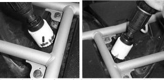
11. Insert the hoses through the holes, cut enough hose to connect the inlet and outlet hoses to the stock hoses you left connected to the ATV.
