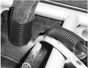
20. Wrap all hoses with the large wire loom and wrap together the overflow bottle lines and wires in the larger wire loom to protect it from cutting and vibration.
