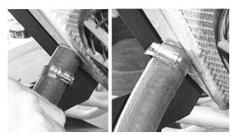
23. Connect the new  $\frac{1}{4}$ " overflow hose to the radiator and to the stock hose using the  $\frac{1}{4}$ " hose barb. We ran the hose along the top of the radiator. Use a zip tie to secure the hose.
