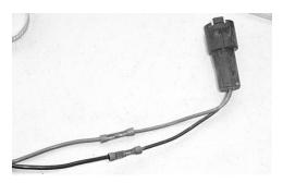
18. Wrap the wires in black tape, and run it through the <sup>1</sup>/<sub>4</sub>" wire loom. Connect the end back to the connector under the plastic,
