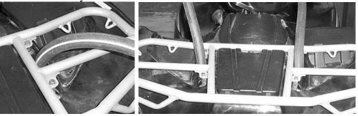
12. Drill one more hole using a 1 <sup>1</sup>/<sub>2</sub> hole saw for the over flow bottle intake and vent lines and the fan wires
