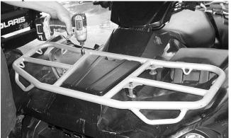
6. Preassemble the new radiator relocating kit. Assemble the frame using the <sup>1</sup>/<sub>4</sub> x <sup>3</sup>/<sub>4</sub> carriage bolts (4ea), <sup>1</sup>/<sub>4</sub> lock nuts (4ea), and <sup>1</sup>/<sub>4</sub> flat washers (4ea).
