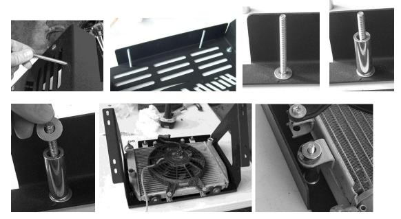
9. Once the kit is assembled, place the kit on the front rack and temporarily mount it to the rack. Next mark the holes that need to be drilled to allow the hoses and wires for the fan to pass through the plastic and rack. Mark all holes and remove the radiator kit from the rack.
