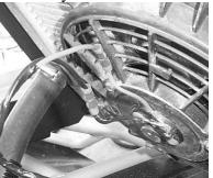
26. Use all zip ties provided in the kit to secure all lines, hoses, and wires so that they do not allow rubbing or touch moving parts.
