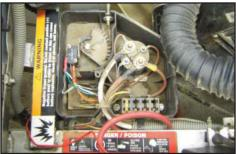
Figure 7 - Remove Solenoid Compartment Cover
