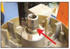
Figure 2 - Snap Ring Removal
