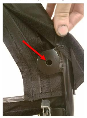
**32.** Locate the mirror mounting bracket on the inside of the door frame. Mark the location of the hole with a punch so that it can be seen on the outside of the door textile.
