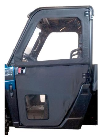
**20.** Move the door into the "closed" position. With the window down, you can make adjustments to the striker bolt and plate to ensure the door fits properly.
