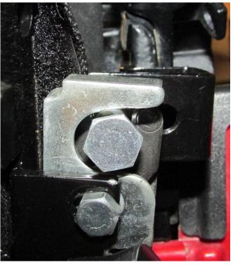
**26.** Shown above is the correct alignment for the striker bolt and latch when the door is fully closed.
