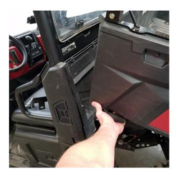
**2.** To install Lower Hinge Plate begin by moving the bed into the dump position. This is done in order to access the factory bolts.
