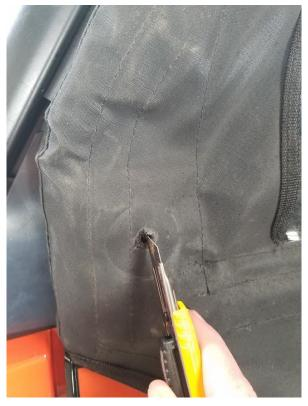
**33.** Using a sharp razor or utility knife, cut the textile so the mirror mounting bolt can pass through.
