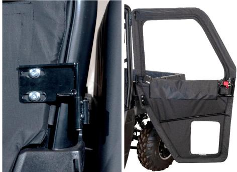
**19.** Insert the Sliding Hinge Pins into the Hinge Mount Barrels and roll down the window for easier adjustment. Rolling down the window will allow you to access and adjust the striker bolt and plate from the outside of the vehicle.
