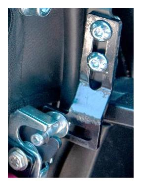
**5.** Attach striker bolt in the remaining slot on the Striker Plate in the orientation shown. Install with supplied nut. (This will adjust how far in and out the door is from the front of the body) (Do not fully tighten at this point.)
