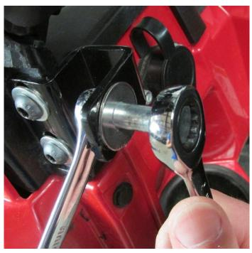
**23.** Open the door and tighten the striker bolt to the plate. Leave the two bolts attached to the ROPS structure loose so that the assembly may move up and down.
