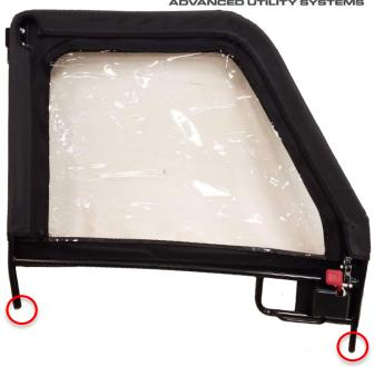
**6.** Locate attachment locations circled on both the Lower and Upper Door Frames. The sleeve tubing in the Upper door frame will slide into the tubing of the lower door frame.
