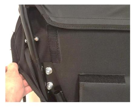
**12.** At the rear of the lower door panel, wrap upper flap tightly around tubing to hook Velcro on the inside of the panel in the area shown.
