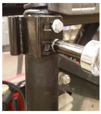
**30**. The Upper Hinge mount plate may be adjusted in and out to affect how much the door will compress the gasket. -Moving this outward, away from the vehicle, should allow the door to close more easily but will not compress the gasket as much.
