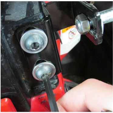
**29.** With the striker bolt in the correct location, fully tighten down the striker bolt to the striker plate and fully tighten the plate to the ROPS Structure.
