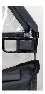
**1.** Align Door frames, ensuring the two pieces are the same side (Both Driver sides, or both Passenger sides. Driver Door shown) and join the two door halves together. It will help to detach some of the Velcro on the lower door frame in order to make access to the tubing easier.
