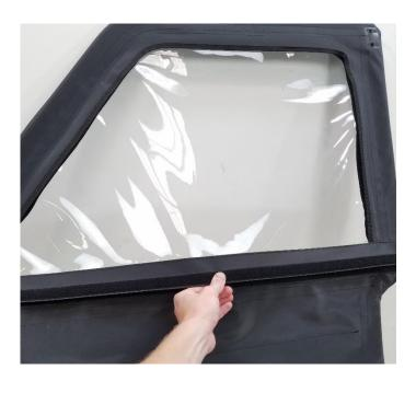
**14.** Pull Upper door textile down firmly and attach to loop Velcro located on the outside of the lower panel as shown.
