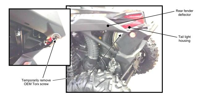
f) Install the rear left fender flare (Item C) to the rear fender deflector using the OEM torx screw removed in previous step.
