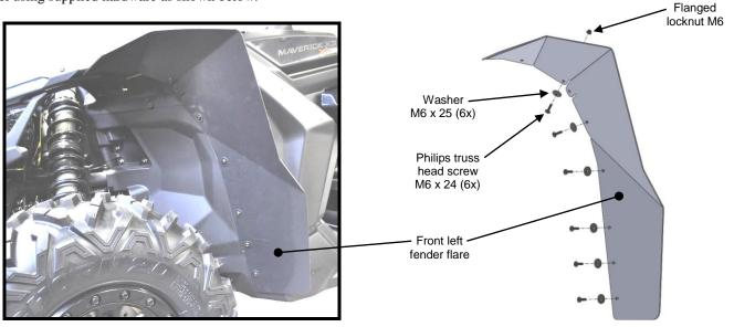
c) Ensure that the front left fender flare is in proper position.
