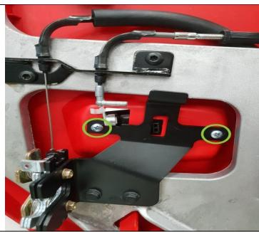
9) Remove the outer panel screws as shown.
