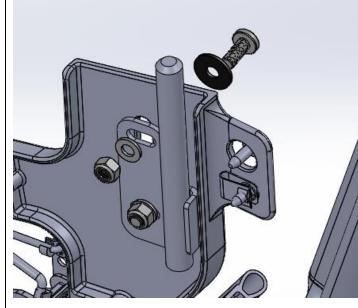
14) Remove the upper front vehicle hinge from the aluminum casting. Save the hardware for use in the next step.
