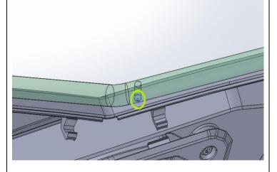
25) Remove the upper door. Install the Jack nut in the marked location.
