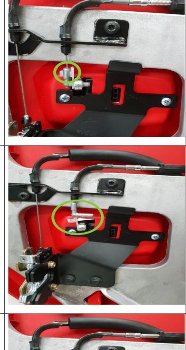
8) Remove the outer handle screws and remove the outer handle.
