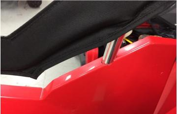
22) Reinstall all plastic panels and handles in the reverse order of removal. Be sure to reconnect all latch cables to ensure correct door operation. The upper door should be easy to install and remove through the holes cut in the previous step.
