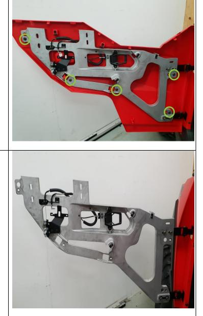
11) Install the front plastic triangle to the lower A-pillar.
