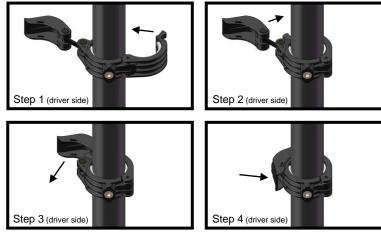
To apply more or less tension to the roll cage, simply rotate the clamp handle from the tension screw as shown below. Over tightening clamps to roll-cage could cause parts failures.
