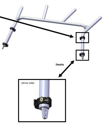
**f**) Install windshield to the clamps as follows without applying final torque. Ensure that all components are properly positioned prior to tightening and properly securing all knobs and all clamps to the roll cage.
