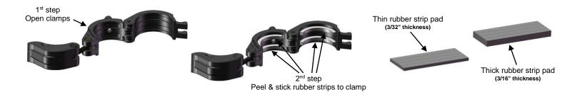
c) Attach the clamps to the roll-cage as shown below and pre-adjust tightening tension of all clamps. NOTE: Keep all clamp handles open as shown in step 3 below; this will allow you to move the clamps up or down when installing the windshield for the first time.
