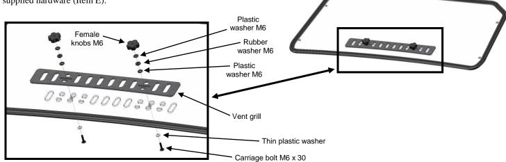
c) Install the windshield to the vehicle using supplied hardware (Item D). Adjust the position of the windshield and tighten. <u>Caution: over tightening any hardware could cause irreversible damage to the windshield.</u>
