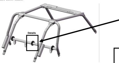
To apply more or less tension to the roll cage, simply rotate the clamp handle from the tension screw as shown below. • Over tightening clamps to roll-cage could cause parts failures.
