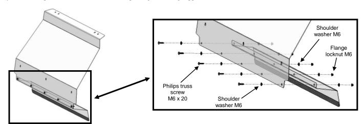
c) Verify "Rubber strip" chart. If required, peel and stick the rubber strips to clamps (Items D) as shown below. Different thicknesses of rubber strips are supplied with the clamp kits in order to fit multiple tube sizes. Make sure that the proper one is used. See chart indicating which rubber strip to use for the different tube sizes. The roll-cage tube size of your vehicle is 1 ¾".
