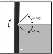
After the first cut, continue installing the bulb seal until the other upper corner (same cut is required).
