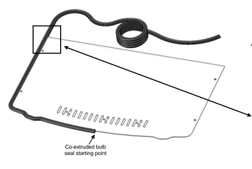
Aligned with the windshield top lip, make a cut of 45 deg. on both sides (do not cut the bulb section, this will cause water infiltrations)
